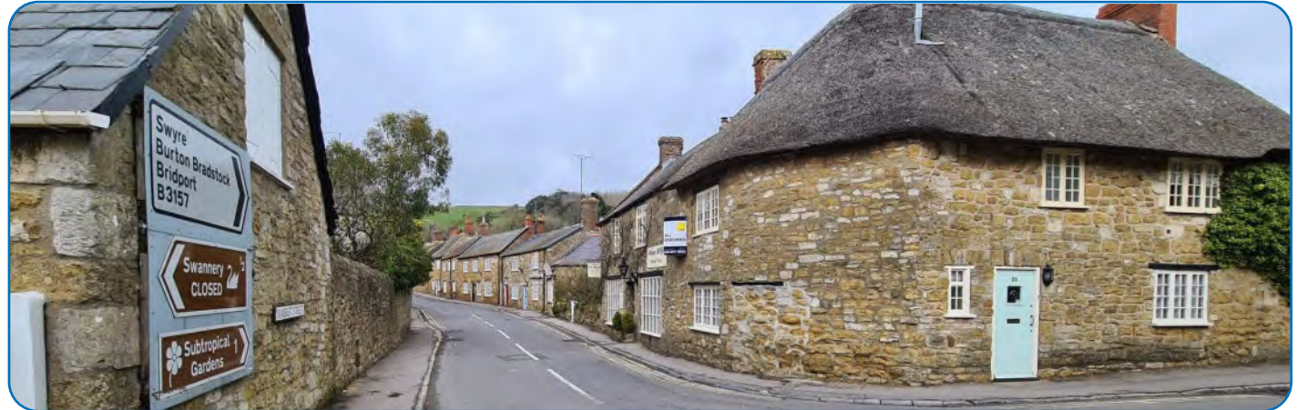
Figure 38: Grade-II listed The Old Post Office - A rubble-stone corner cottage with rounded corner. Thatch roof with rounded hip to corner with Market Street
