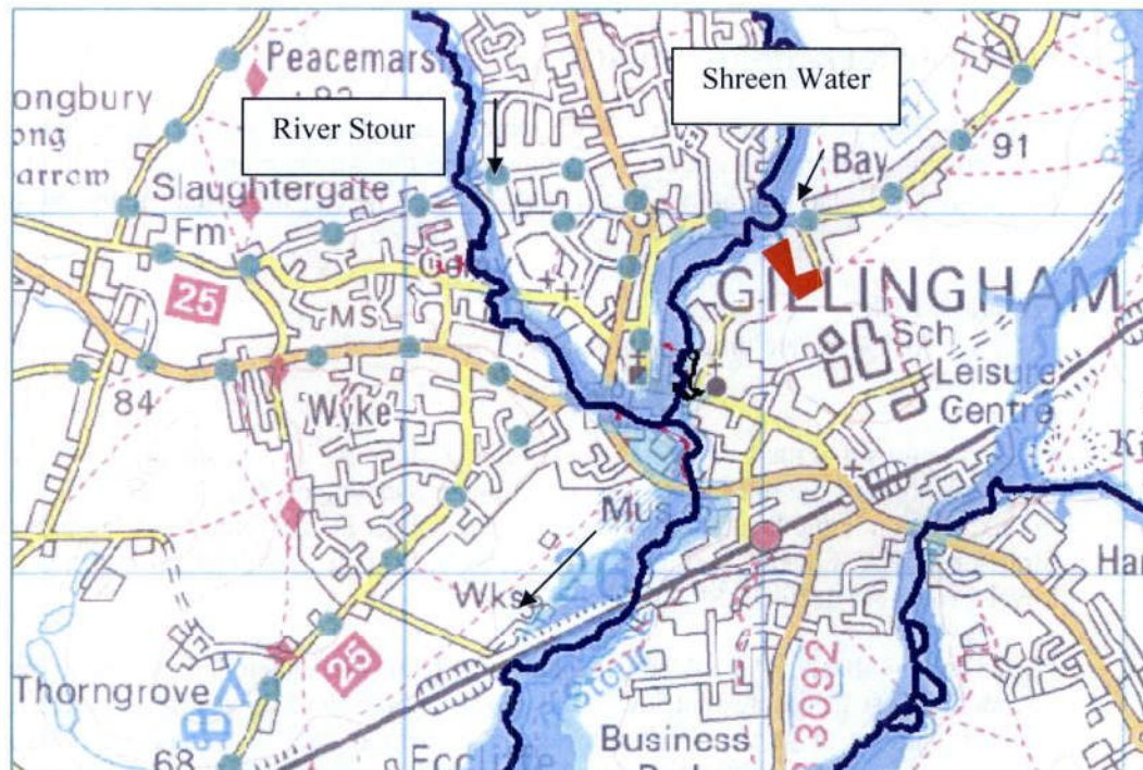
EA Output: Extent of flooding in Gillingham (site shown in red) (dark blue high risk and light blue medium risk)
