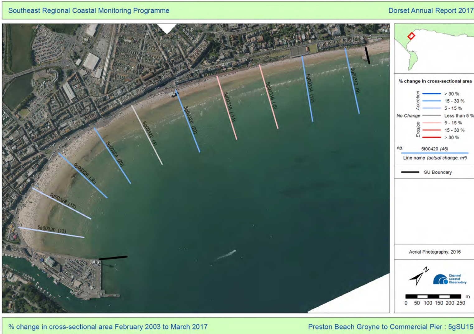
Figure 2-9 CSA changes for profiles monitored as part of the SERCMP between spring 2003 and spring 2017 for the area between Greenhill Groyne and the Pavilion Peninsula (from Channel Coastal Observatory, 2017).
