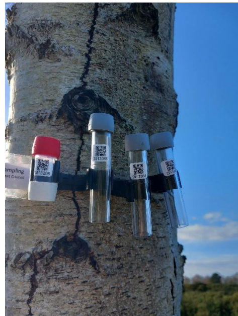
Figure 12 Air Sampling diffusion tubes
