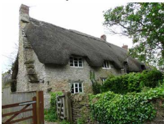
Figure 21: Yew Tree Cottages: Row of three Grade II listed terraced cottages featuring a coursed rubble-stone wall, thatched roof with gable ends, wooden casement windows and glazing bars and prominent protruding chimneys at either end.
