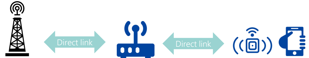
5G router enabling connection of non-5G enabled devices to the 5G network
