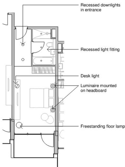
Figure 5 - Typical bedroom lighting layout, provided by the architects.
