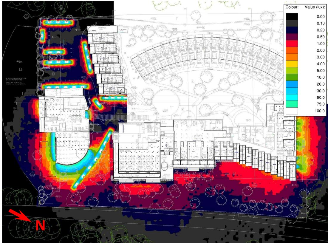
Figure 7 - False colour lux plot, site plan view.
