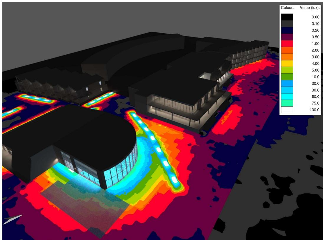
Figure 9 - False colour lux plot, view from the south-east.
