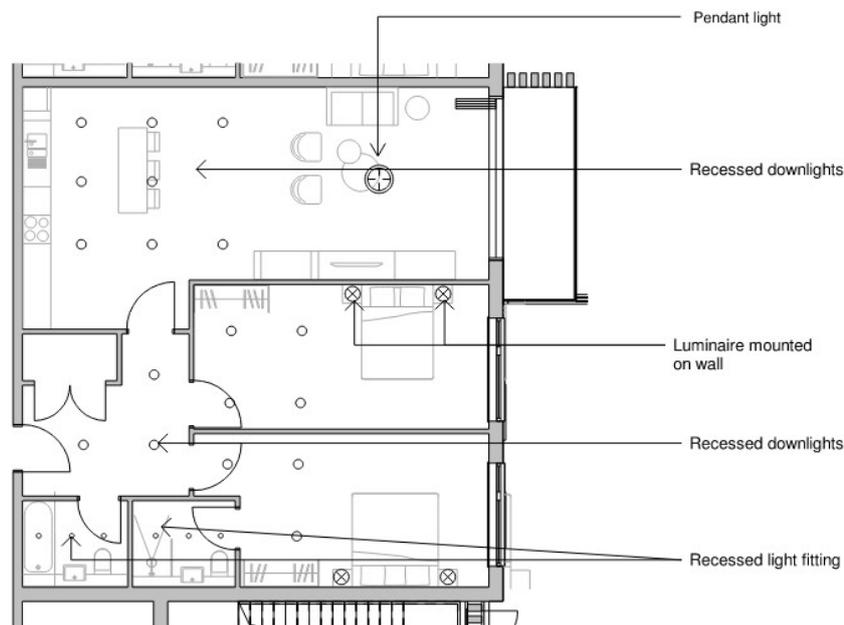
Figure 6 - Typical apartment/villa lighting layout, provided by the architects.
