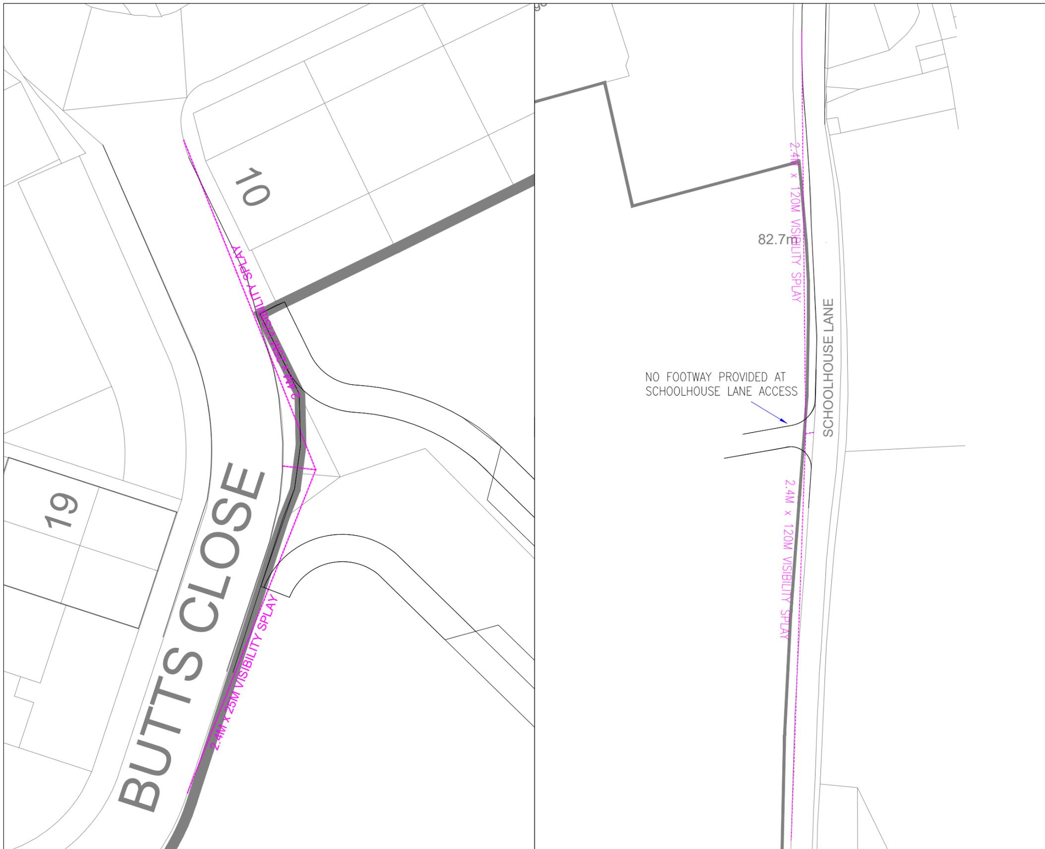
BUTTS CLOSE 2.4M x 25M SITE ACCESS VISIBILITY SPLAY (SCALE 1:250)
