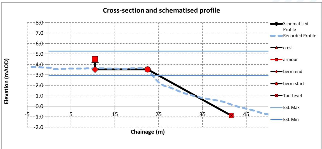
**Figure 4-3: Neural Network Schematisation, Example Profile 4, Baseline Scenario**
