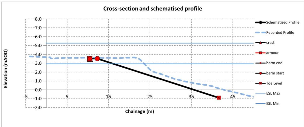
**Figure 4-5: Neural Network Schematisation, Example Profile 4, Undefended Scenario (compare to Figure 4.3 with defence).**
