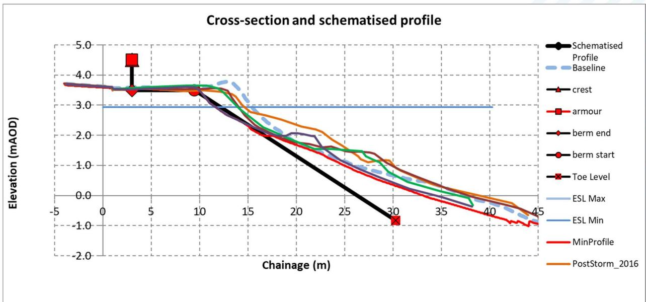
**Figure 4-6: Neural Network Schematisation, Example Profile 5, Eroded Beach Scenario**
