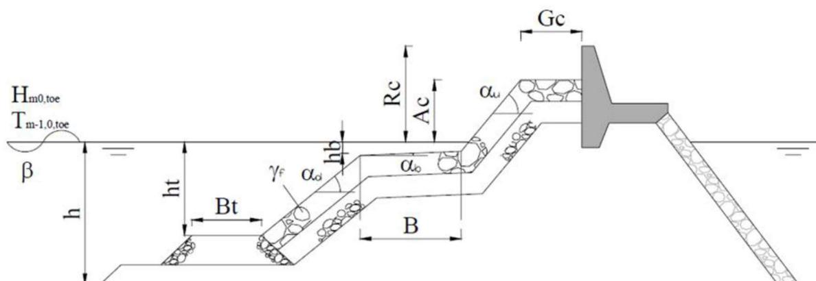
**Figure 4-1: Schematisations of a typical beach profile for analysis using the Neural Network overtopping tool (Source: EurOtop manual)**
