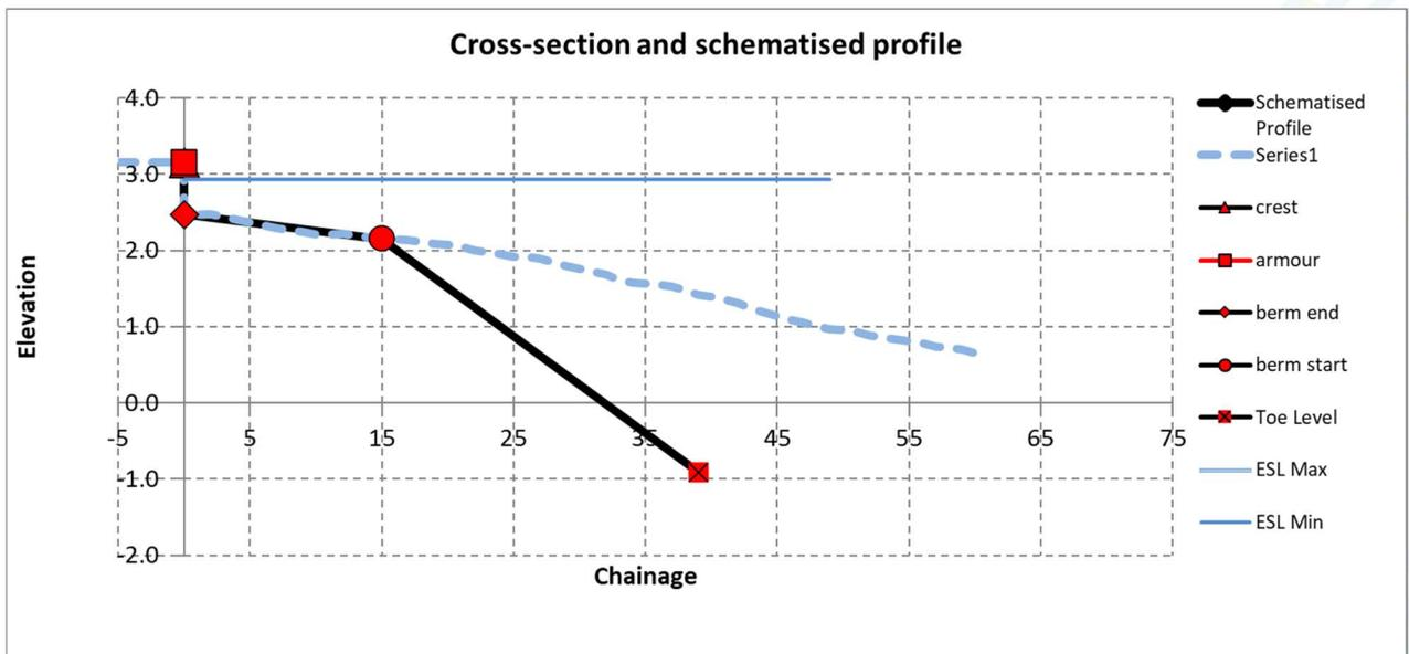
**Figure 4-2: Neural Network Schematisation, Example Profile 1, Baseline Scenario**
