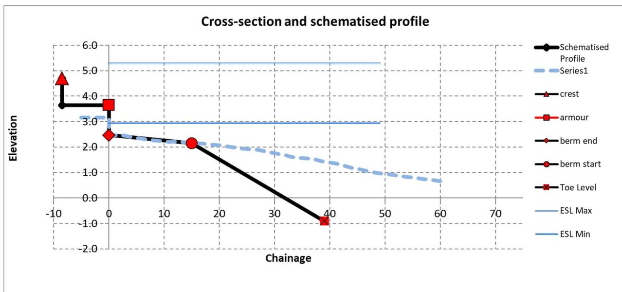
**Figure 4-7: Neural Network Schematisation, Example Profile 1, Future Defence Scenario.**
