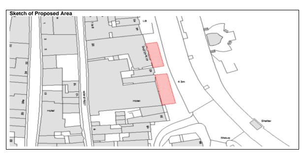
Area of Highway to be Occupied (i.e. 4.0m x 2.5m): 20m x 6.5m and 16m x 6m
