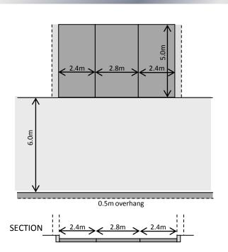
Parking bays for disabled people are designed so that drivers and passengers, either of whom may be disabled, can get in and out of the vehicle easily. They allow wheelchair users to gain access from the side and rear.
