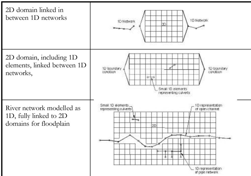
Figure 8.3 - Overview of 'typical' 2D model development
