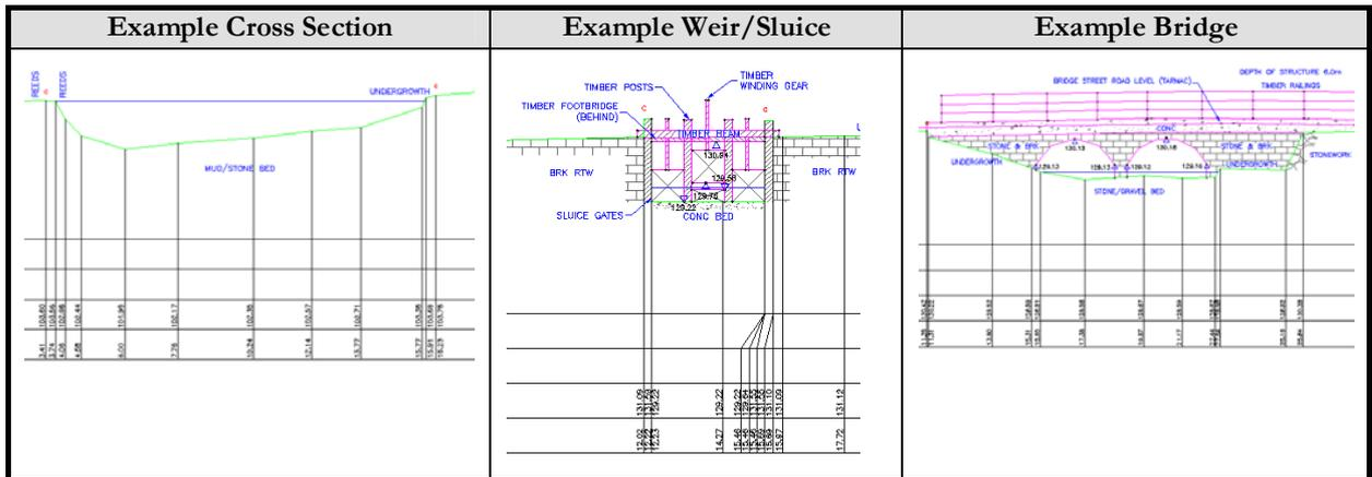
Figure 8.4: Example Channel Survey Data
