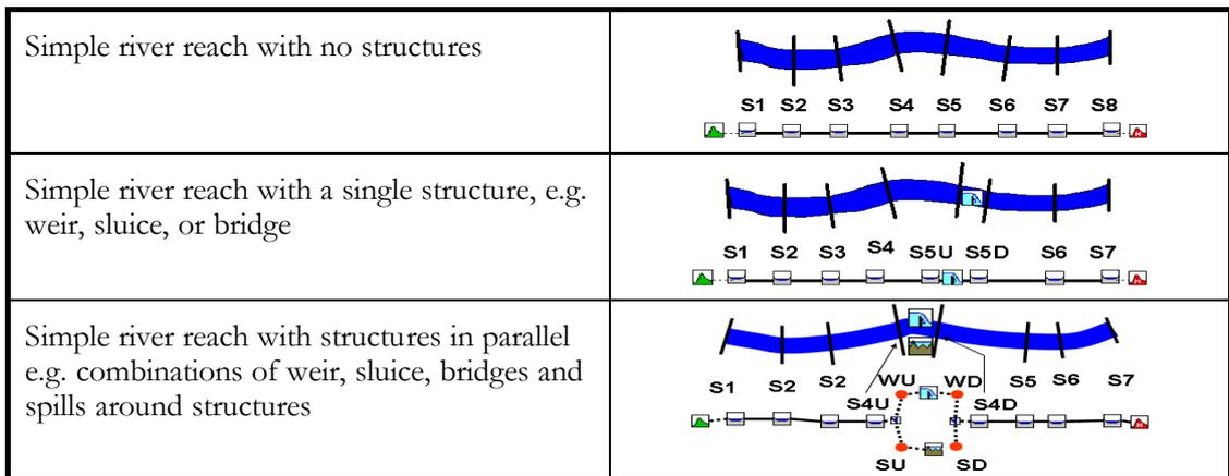
Figure 8.2 - Overview of ‘typical’ 1D model development
