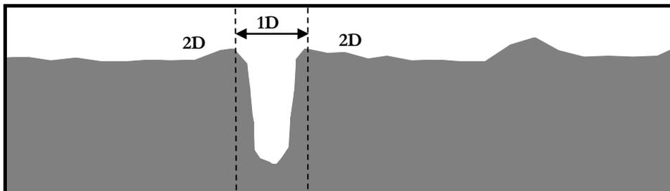
**Figure 8.1 - Modelling a river channel in 1D & floodplain in 2D**
