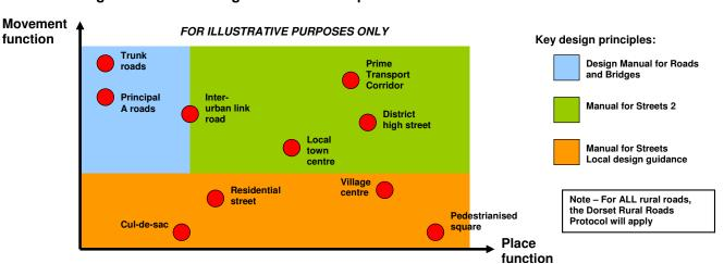
Figure 7.1 Considering the functions of place and movement in road hierarchies
