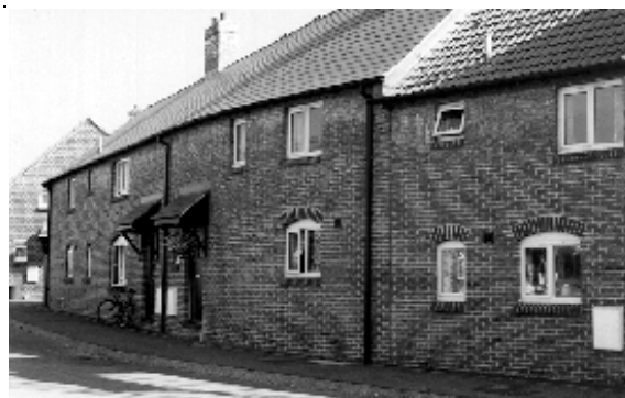
Village housing, recently constructed at Cranborne, comprising short terraces which follow the alignment of the street. Good solid/void relationship between wall area and irregularly-placed. Colour and textural contrasts achieved by roof materials.
