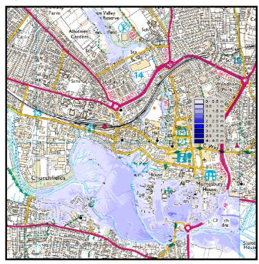
Figure 6.6 Variation in flood depth for the River Avon, Nadder, Bourne and Wylye at Salisbury
