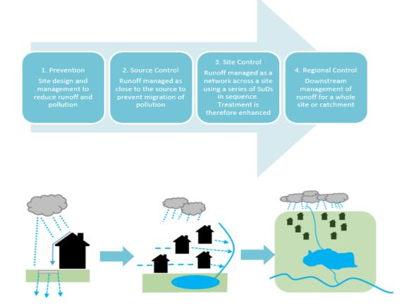
SuDS components should be selected based on design criteria and how surface water management is to be integrated within the development and landscaping setting. By using a number of SuDS features in series it is possible to reduce the flow and volume of runoff as it passes through the system as well as minimising pollutants which may be generated by a development.
