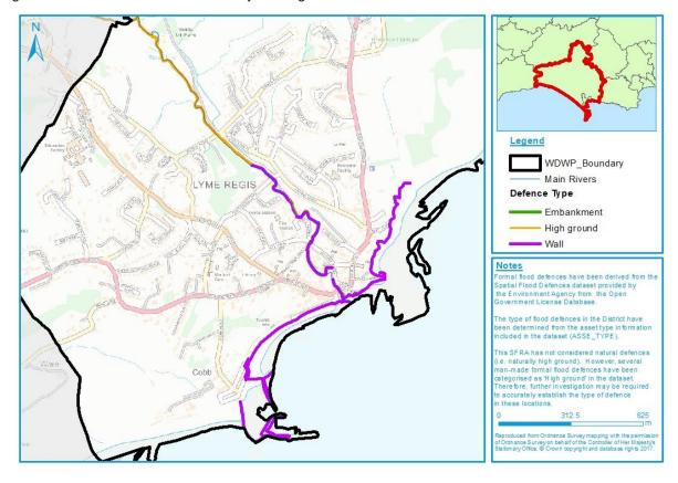
Figure 6-17: Design Standard of Protection for defences in Lyme Regis
