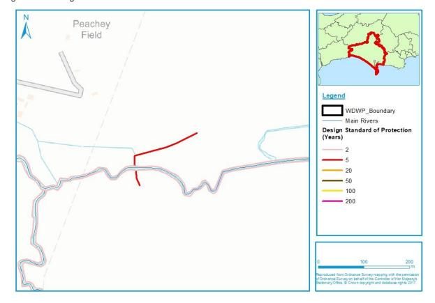
Figure 6-5: Design Standard of Protection for defences in Bradford Abbas
