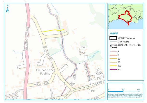
Figure 6-15: Design Standard of Protection for defences in Cerne Abbas
