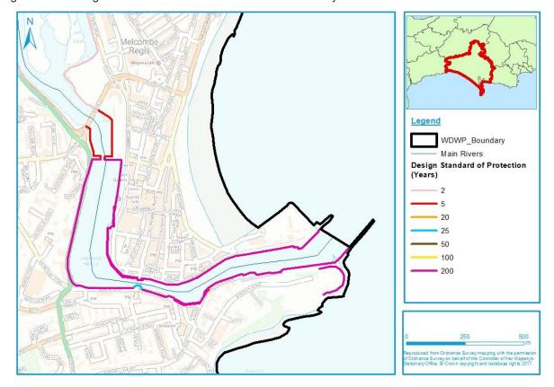
Figure 6-27: Design Standard of Protection for defences in Weymouth
