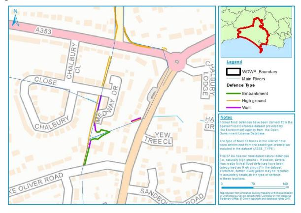
Figure 6-21: Design Standard of Protection for defences in Preston
