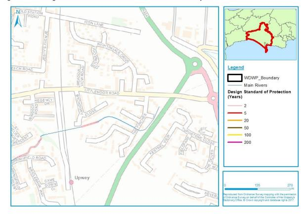
Figure 6-11: Design Standard of Protection for defences in Broadwey
