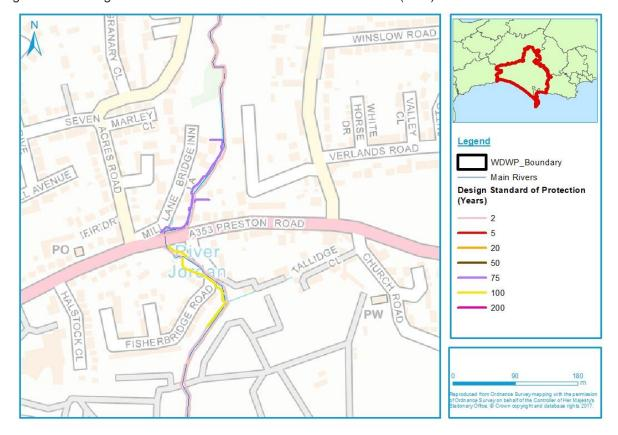
Figure 6-23: Design Standard of Protection for defences in Preston (East)
