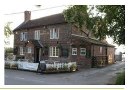
(brick (Flemish bond with flared headers), tiled roof with gable ends, stone copings)
