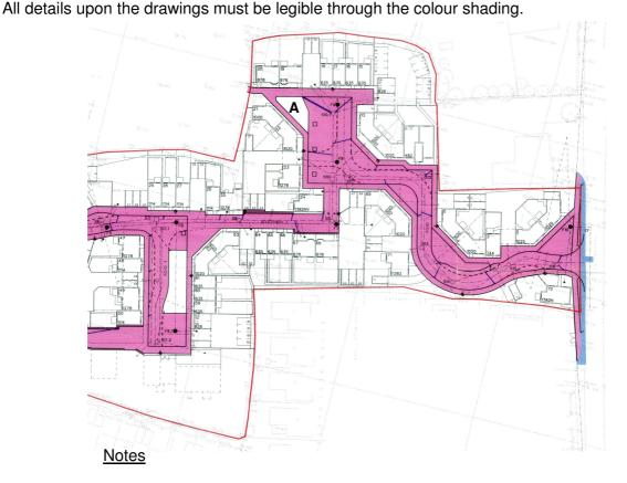
In this example, only the gullies and spurs to the main carrier drain are to be adopted by the Highway Authority. The main carrier drain is a public surface water sewer to be adopted by the appropriate water company.
