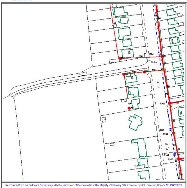
WATER MAINS Public Private Abandoned Raw Water Private/ **SEWERS Public** Section 104 Foul Combined Surface Rising Main Culverted Water Course Highway Drain Effluent Disposal Main
