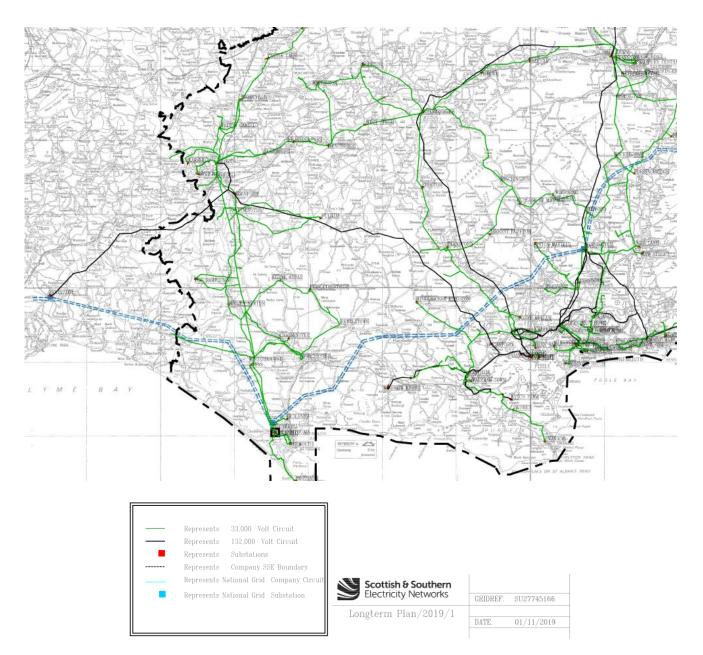
Figure 6 – SSEN Long Term Plan Electricity Network covering Dorset County, Showing Network Topology for 33kVand 132kV.
