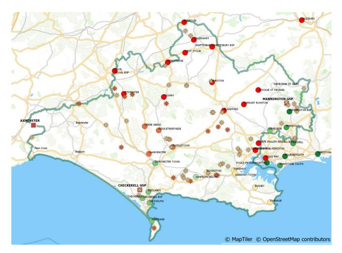
Figure 32 – DFES Projected Substation Generation Headroom (2040) and Proposed Solar PV Locations
