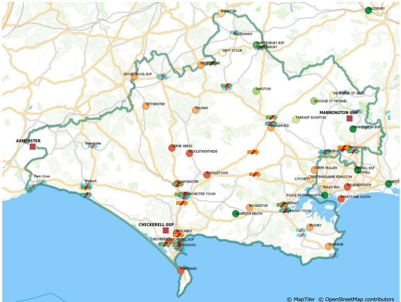
**Figure 20 - Dorset Planned and Probable Public and Council EV Charging Locations and Substations with Headroom Indicators for 2030**
