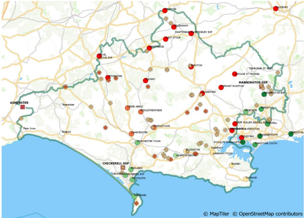
**Figure 32 – DFES Projected Substation Generation Headroom (2040) and Proposed Solar PV Locations**
