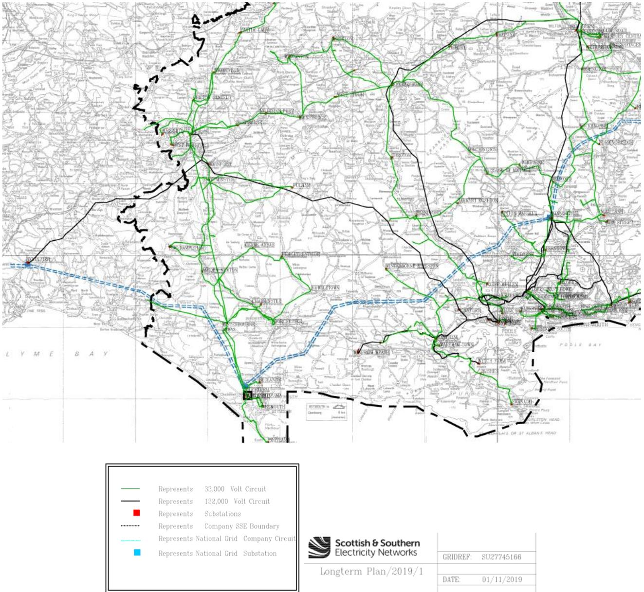
**Figure 6 – SSEN Long Term Plan Electricity Network covering Dorset County, Showing Network Topology for 33kV and 132kV.**
