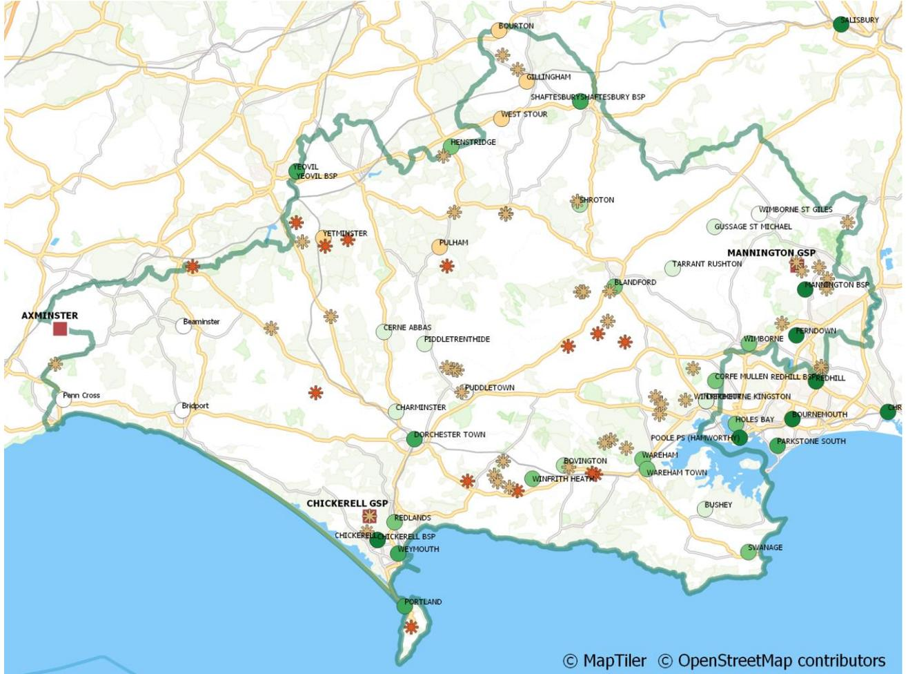
**Figure 31 – DFES Projected Substation Generation Headroom (2030) and Proposed Solar PV Locations**
