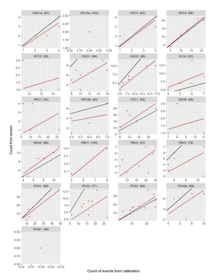
Figure 15: Linear regressions between counts from the sensor and the number of 'events' observed during calibrations. Each red dot indicates the result from a single calibration, fitted with a red line indicating the linear regression (with intercept set to zero). The black line indicates a line of 1:1 (line of equality).
