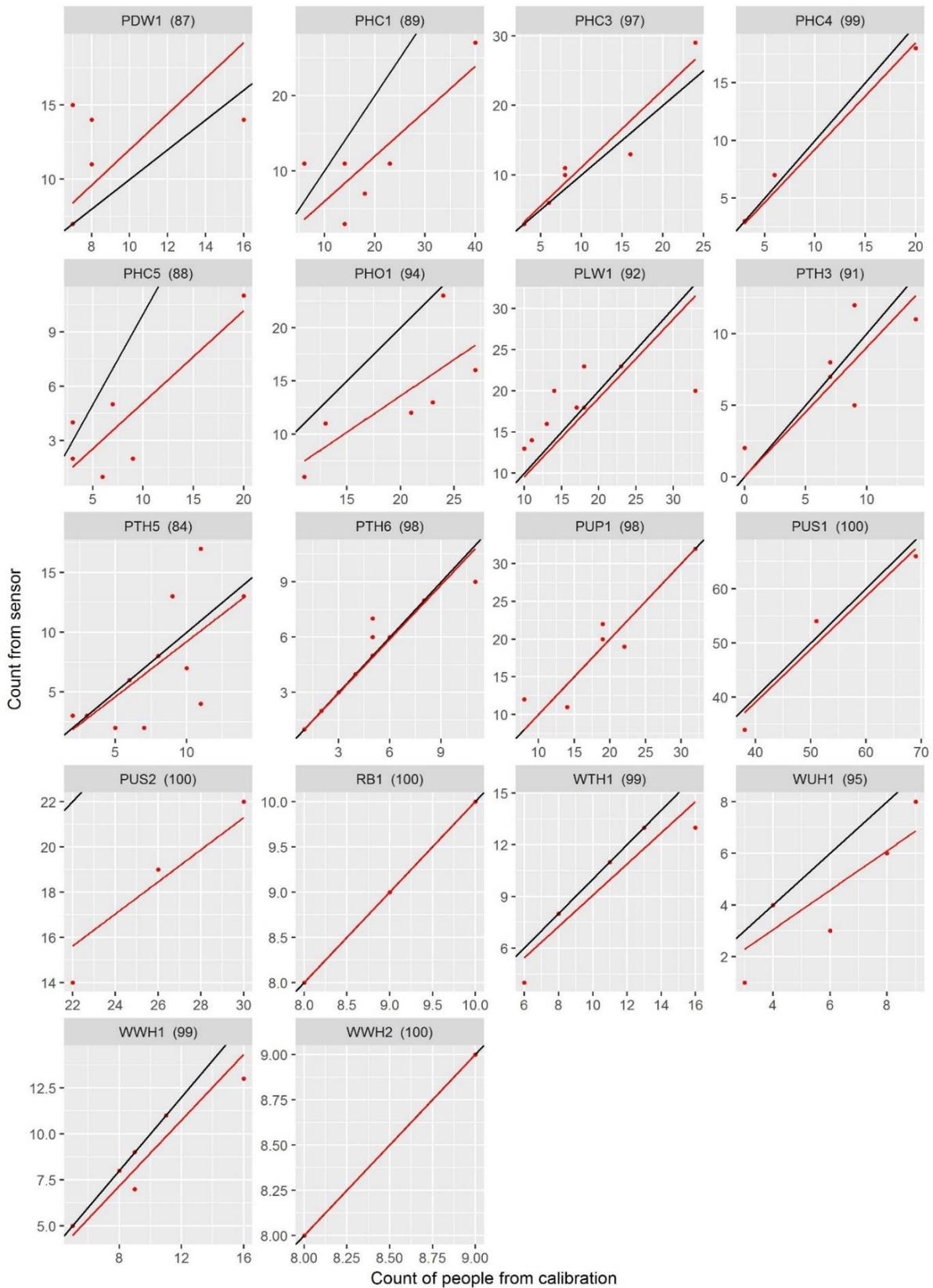
**Figure 19: Linear regressions between counts from the sensor and the actual number of people observed during calibrations. Each red dot indicates the result from a single calibration, fitted with a red line indicating the linear regression (with intercept set to zero). The black line indicates a line of 1:1 (line of equality).**
