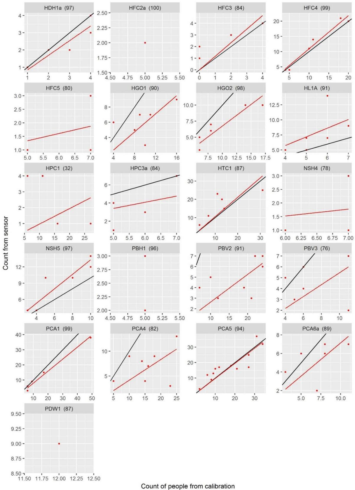
**Figure 18: Linear regressions between counts from the sensor and the actual number of people observed during calibrations. Each red dot indicates the result from a single calibration, fitted with a red line indicating the linear regression (with intercept set to zero). The black line indicates a line of 1:1 (line of equality).**
