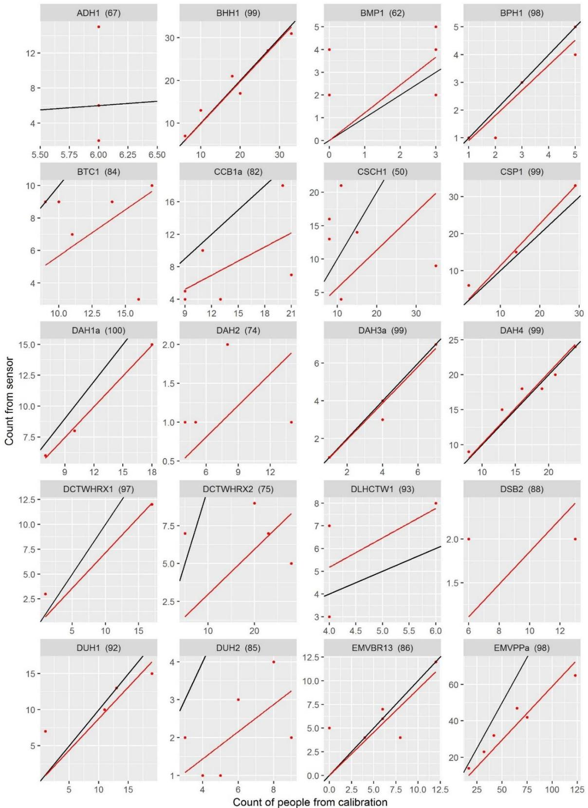
Figure 17: Linear regressions between counts from the sensor and the actual number of people observed during calibrations. Each red dot indicates the result from a single calibration, fitted with a red line indicating the linear regression (with intercept set to zero). The black line indicates a line of 1:1 (line of equality).
