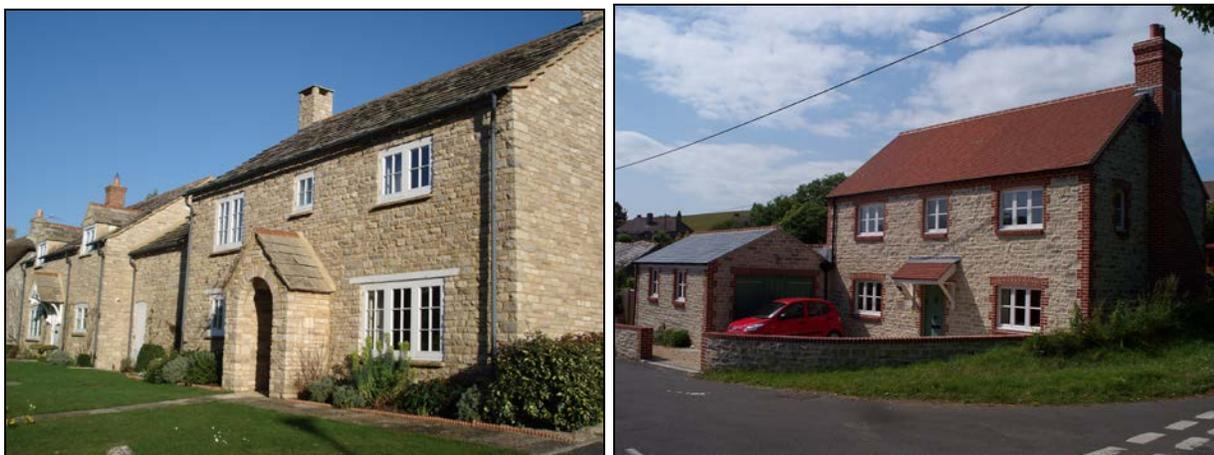
*Purbeck stone in new build at Corfe Castle (left) and West Lulworth (right). Recent housing schemes which largely follows a traditional theme. Note use of newly manufactured stone roof tiles in the Corfe scheme, and careful use of bricks to define edges in the Lulworth scheme.*
