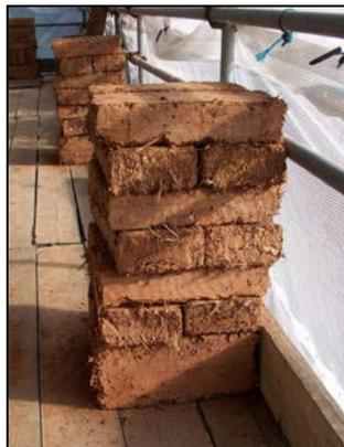
*Cob blocks. These can be used like bricks in new build and repairs to existing cob walls. The blocks are joined using lime mortar.*
