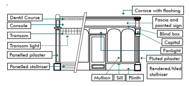
Above: Generalised details for the two most common standard types. There will be many cases where the detailing of historic examples differs from the schemes shown, however the basic components and principles of design are fairly consistent. Above left: parade type. Above right: free standing type – see also detail below left. Below right: mullion detail. Note the beading is always on the inside.
