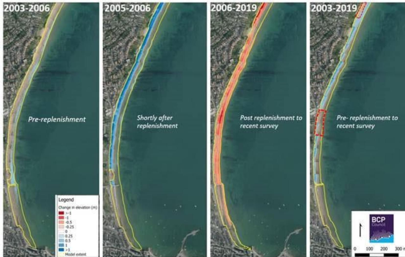
Figure 2-6 Topographic elevation difference plots 2003 until 2019 – showing pre replenishment, shortly after replenishment, change since the replenishment and change pre replenishment to recent (with the red-dashed lines highlighting erosion hotspots).
