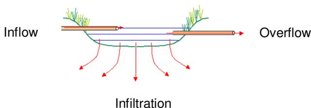
Figure 4.3d - Cross-section of a Pond
