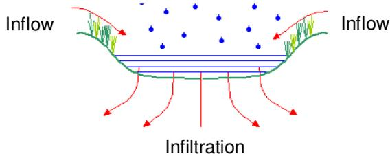
Figure 4.3b - Cross-section of a Filter Strip
