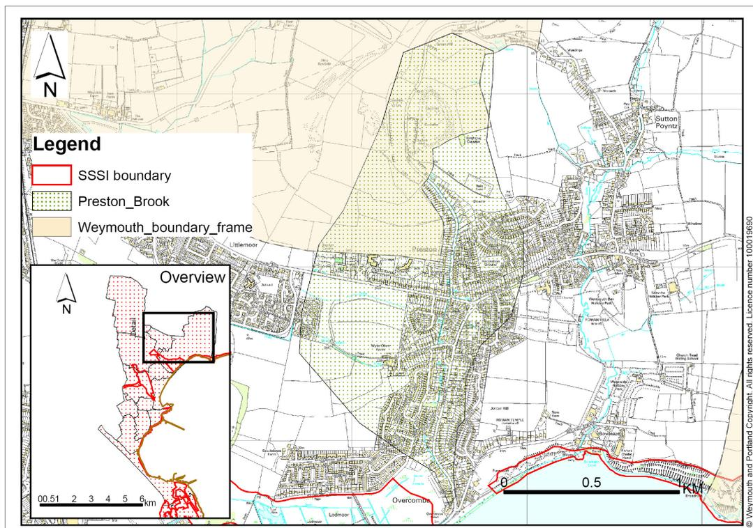
HEC-RAS hydraulic modelling was used to estimate peak water levels along the Preston Brook for a range of flows to determine the viability of flood alleviation options which resulted in channel improvements, raising the standard of protection to 1 in 25 years for properties within the study area.
