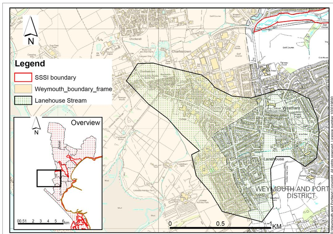
A hydrological study was carried out, followed by HEC-RAS hydraulic modelling. The HEC-RAS modelling highlighted the insufficient capacity of the culverts downstream of Lanehouse Rocks Road. New developments therefore need to implement Sustainable Drainage systems (SUDS) to minimise the affect of the development on the downstream flood risk and to ensure the problem is not moved downstream.
