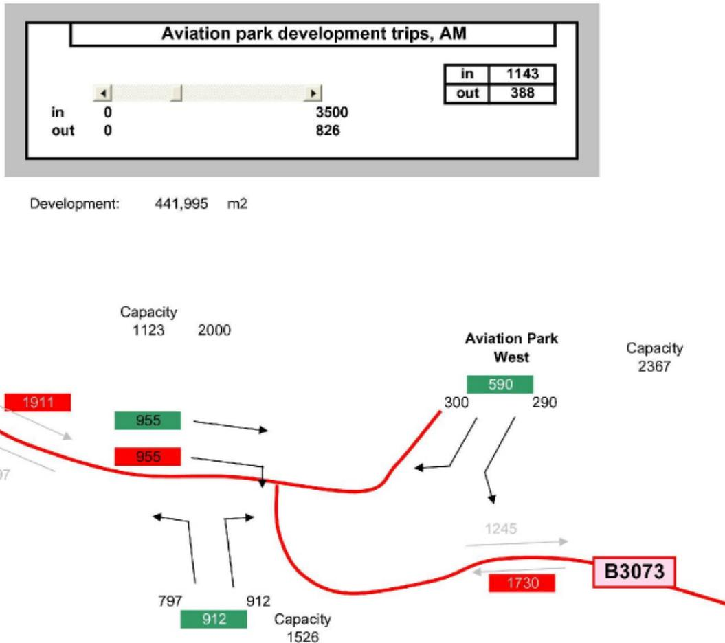
Figure 3.9: Final predicted position - AM peak - Chapel Gate junction
