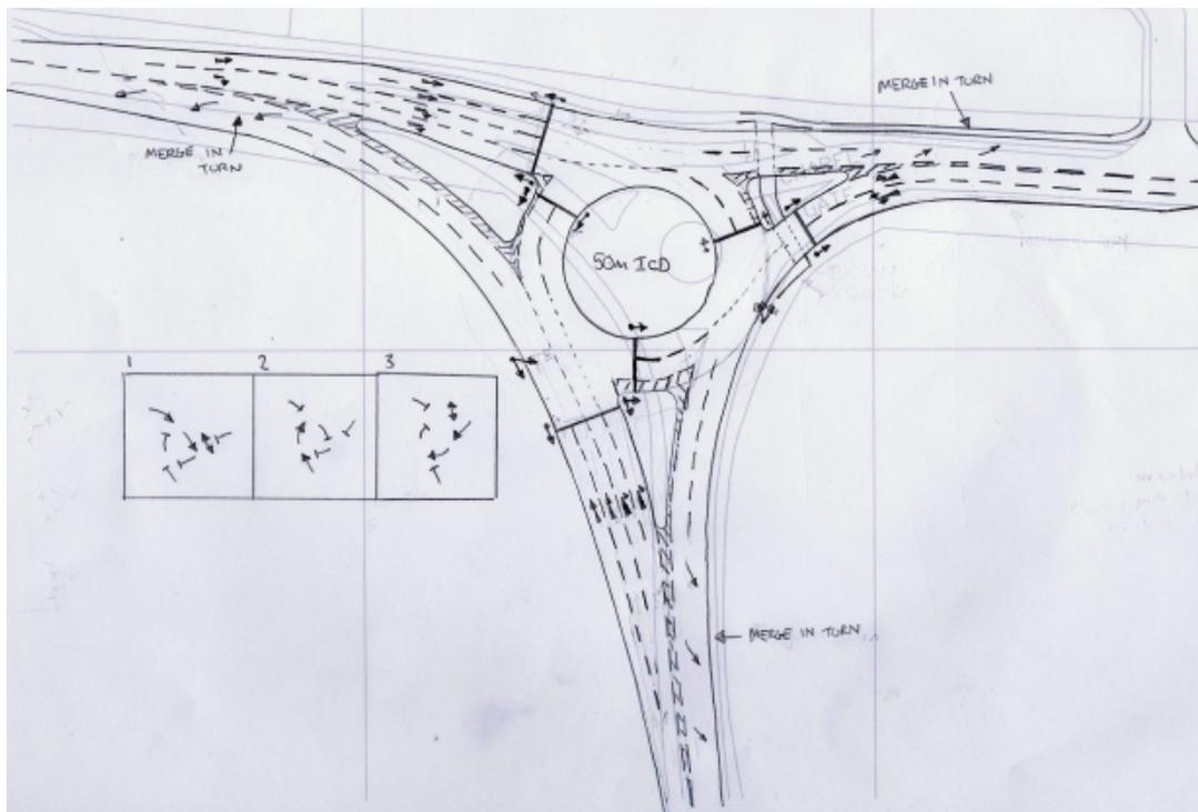
Figure 5.1 - Proposed Signalised Roundabout at Chapel Gate
