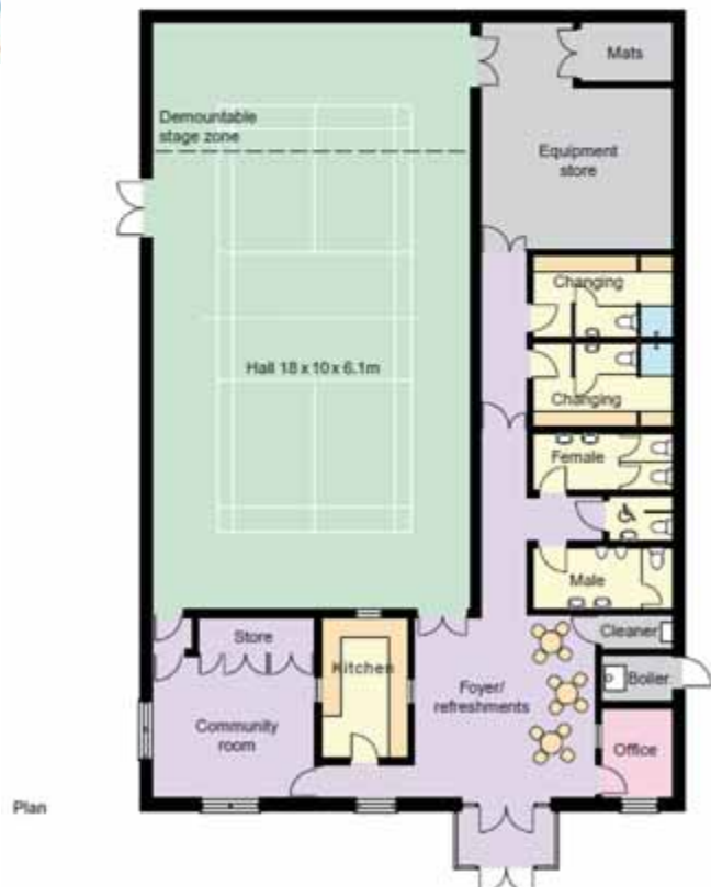
Plan and section of an economically designed hall layout. The double set of corridor doors would allow the changing rooms to be used for stage productions.
