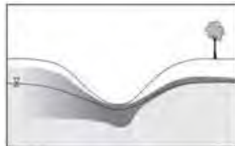
Figure 4 – Illustration of topographic impact on aquifer (Ref: BGS Technical Report WD/97/34)
