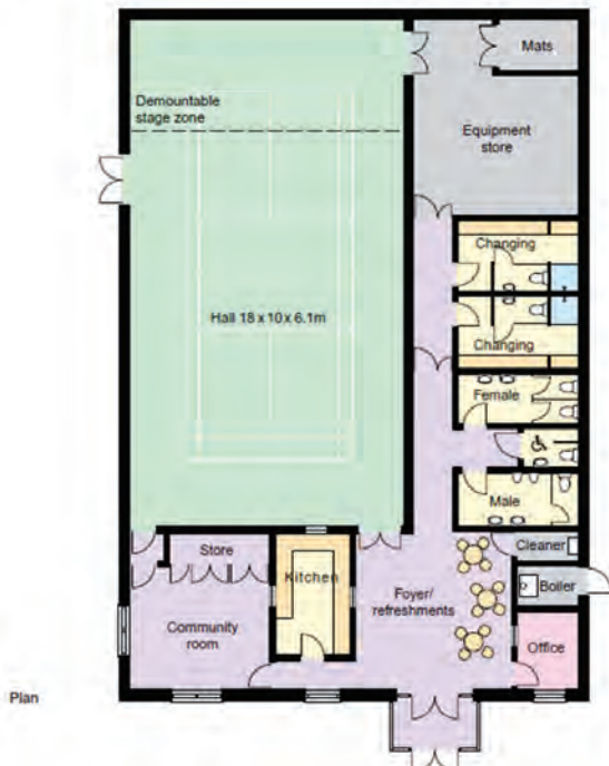
Plan and section of an economically designed hall layout. The double set of corridor doors would allow the changing rooms to be used for stage productions.
