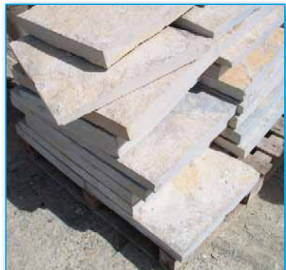
Newly prepared Purbeck stone paving
